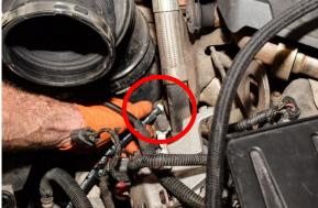
Step 15: Install the provided piece of hose over the stud for the CAC boot clamp where the first hose runs past.
