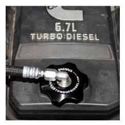
Step 20: Start the engine and check all the hose connections for leaks. Tighten all the fittings, if necessary, then recheck.
