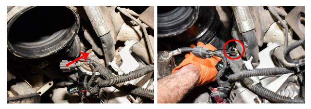
Step 3: Wrap threads on brass elbow with thread tape and install elbow into the oil filter housing with the outlet pointed towards the right headlight. \*\*You may need to loosen but not remove the lower bolt (pictured) for the coolant tube mounting bracket, then using a prybar gently pry the tube towards the front of the truck to give you enough clearance to install the brass elbow.
