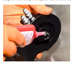
Step 7: Install the Amsoil Filter adapter onto the filter adapter then tighten with a 19mm wrench or adjustable wrench.
