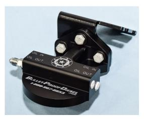
Step 9: Attach the hoses to the filter adapter and tighten. The 39" hose connects to the "oil in" port and the 58" hose connects to the "oil out" port. \*Be sure to use **two** wrenches.
