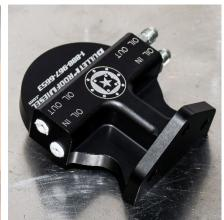
Step 6: Put a couple drops of red thread locker onto the threaded port on the bypass oil filter adapter.
