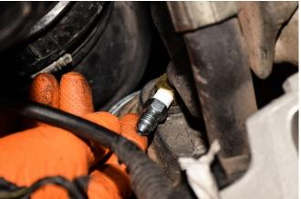
Step 5: Apply the thread sealing tape to both fittings and pipe plugs then install into the oil filter adapter.
