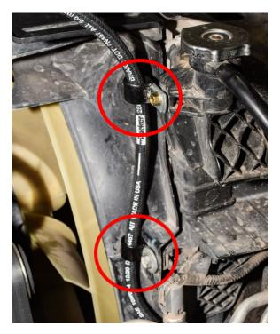
Step 17: Route the remaining section of the 58" hose towards the oil fill cap.
