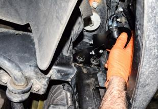
Step 12: Tighten the frame bolts onto the mounting bracket and install the oil filter.
