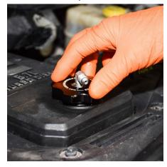
Step 19: Attach the oil line to the fitting on the oil fill cap using two wrenches to ensure a snug fit.
