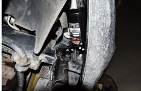
Step 13: Pull both hoses up and out of Grill area then pass both hoses through the core support and over the top of the intercooler pipe.
