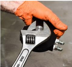
Step 8: Using the supplied hardware, attach the assembled filter adapter to the mounting bracket and tighten hardware.
