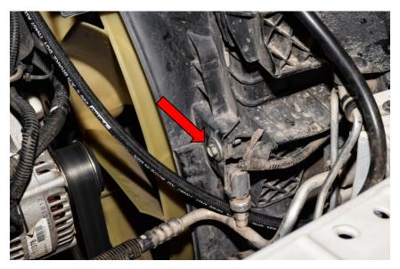
Step 17: Attach the rubber dipped loop clamps to the hose and then attach the clamps to the fan shroud. Reuse existing screw to mount lower clamp. Install upper clamp using supplied hardware as shown.
