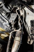
Step 14: Route the 39" hose from the "Oil In" port of the bypass filter adapter along the intercooler pipe to the fitting that was installed on the engine oil filter housing. Attach the hose to the fitting and tighten.
